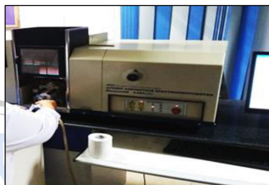
Figure 2: Sample analysis at AAS 4141
